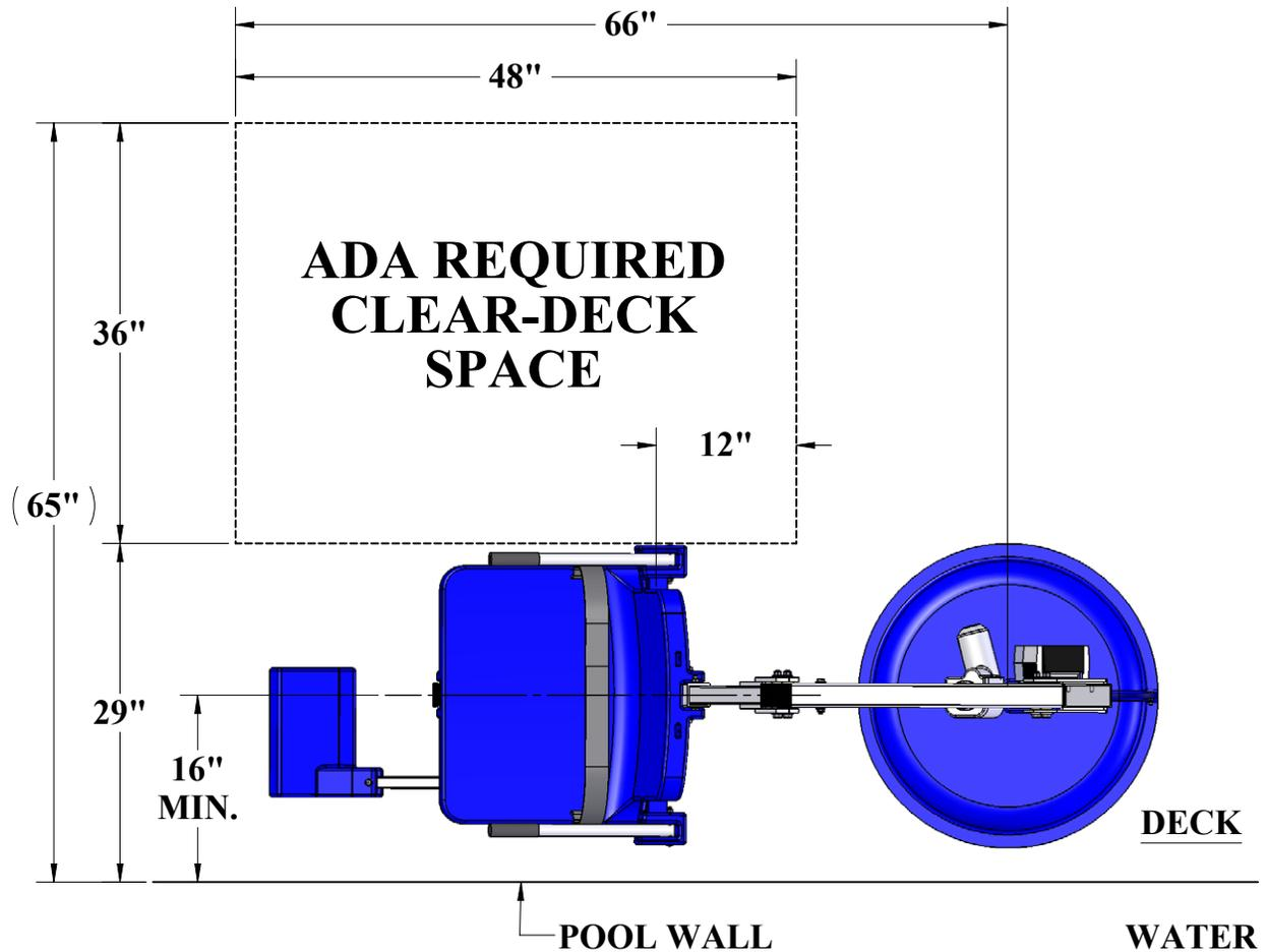
Before installing the TITAN Lift it will be necessary to select a location for the anchor. The versatility of the TITAN Lift allows it to be installed in a wide variety of locations, but the owner/installer should be aware of the requirements of the Americans with Disabilities Act (ADA) with concern to lift installations. The diagram above shows an example of an ADA compliant installation, which incorporates the following ADA rules in order to be compliant:
