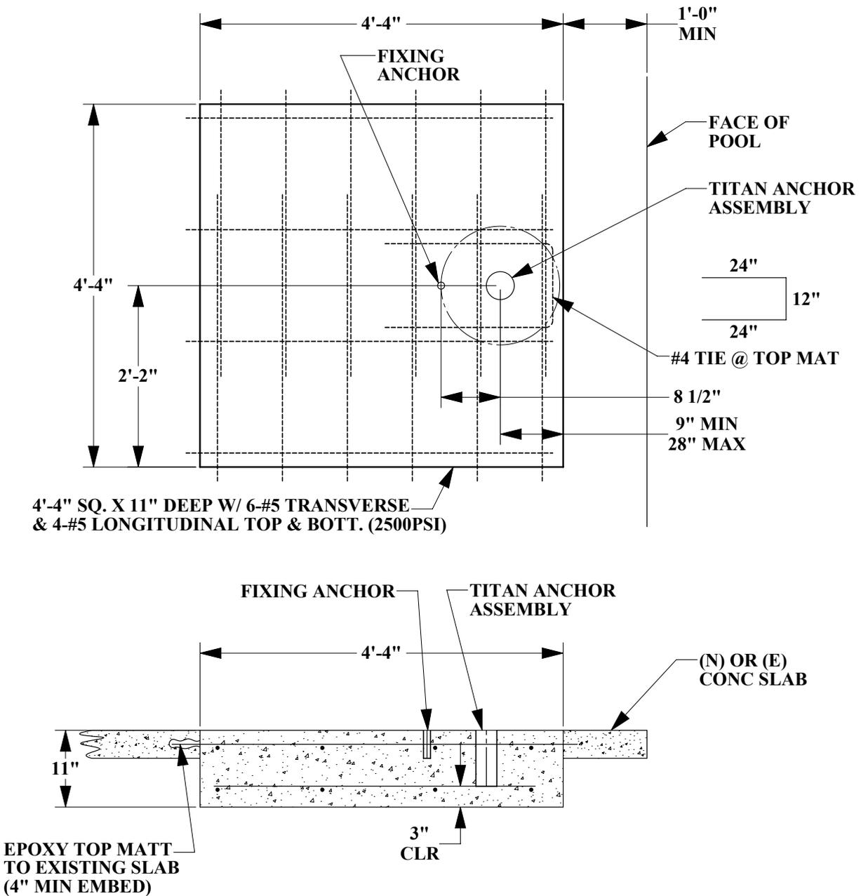
**NOTE: For the SLING OPTION the maximum setback distance (from the pool wall to the anchor) is 24".**
